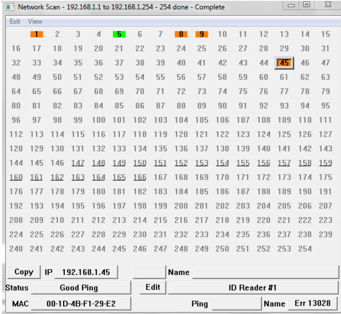
As a minimum, the scan should show each of the card readers in the system and the address of the Corsair computer. If the scan does not work network Firewall settings may need to be changed.
